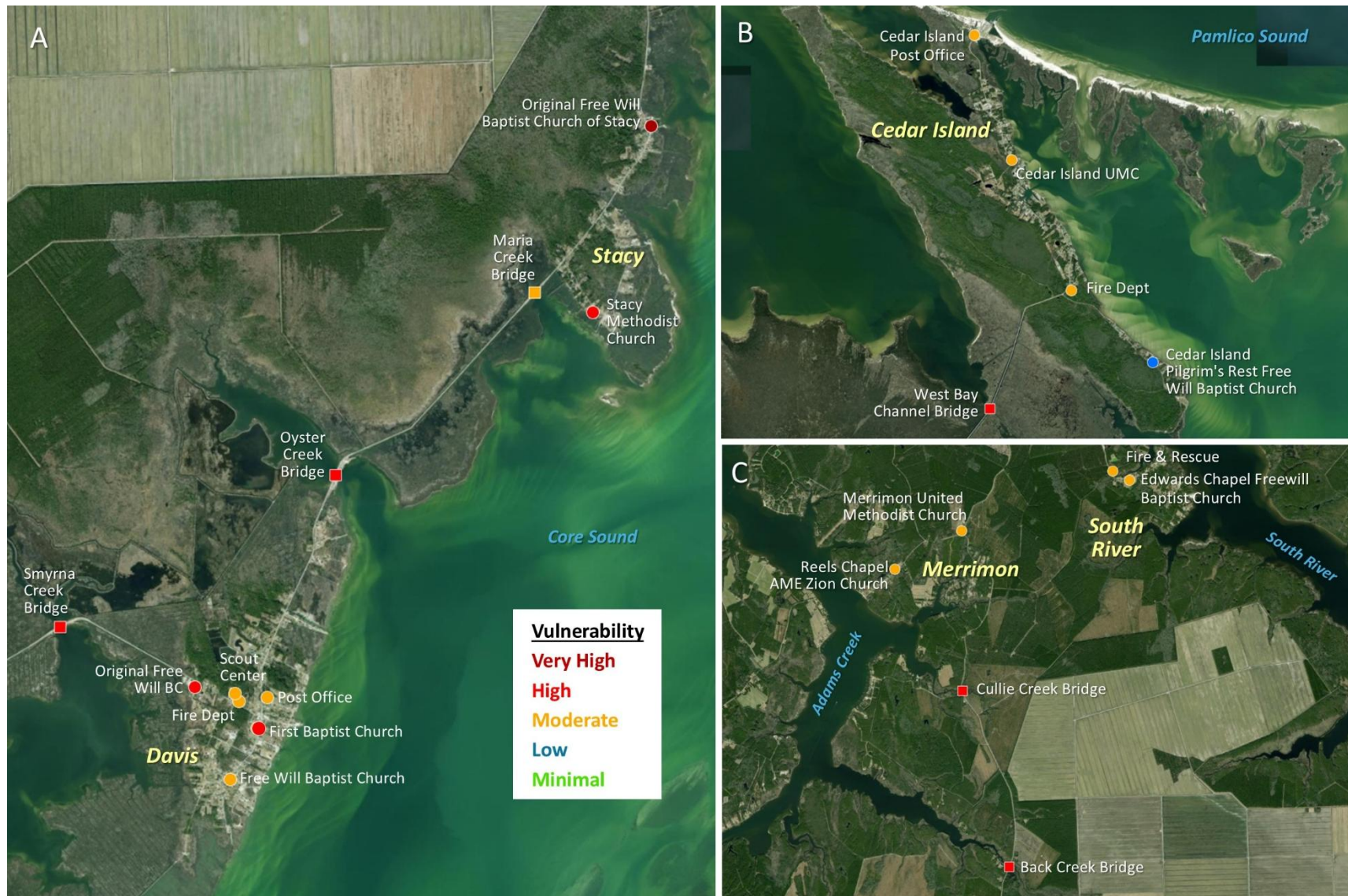
Figure 18. Vulnerability results for A) Davis and Stacy, B) Cedar Island, and C) Merrimon and South River. Buildings are represented by circles and bridges by squares.
